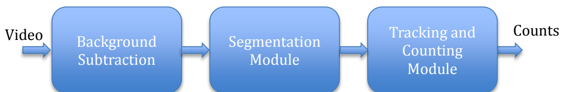
Figure 2: Block diagram of vehicle tracking architecture
